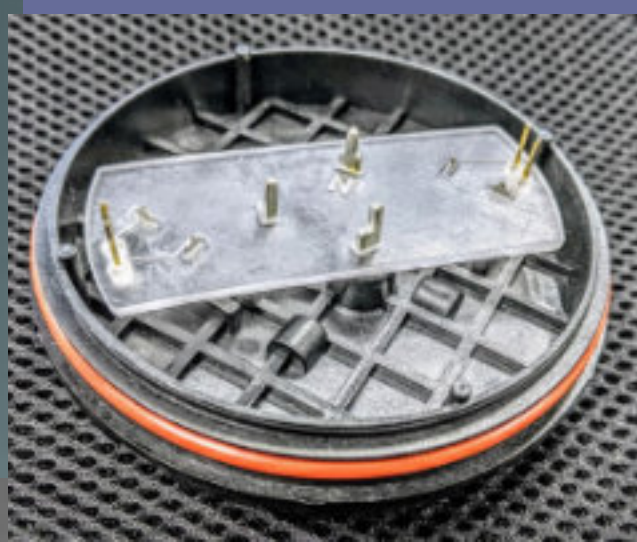
Above: 3D printed insert shows reconfiguration of the power ports
