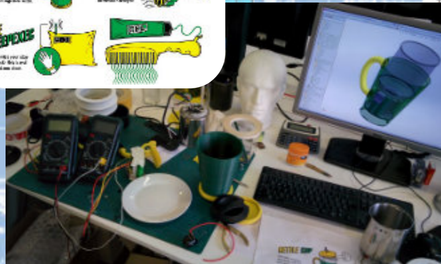
The Handle 3D Printed Yellow ABS with rivet inserts
